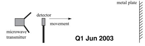
A microwave transmitter directs waves towards a metal plate. When a microwave detector is moved along a line normal to the transmitter and the plate, it passes through a sequence of equally spaced maxima and minima of intensity.
