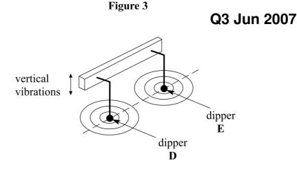
Figure 3 shows two dippers, **D** and **E**, mounted on the same vibrating beam. The dippers touch the surface of the shallow water in a ripple tank. When the beam vibrates, waves travel outwards in all directions on the surface of the water from each dipper.
